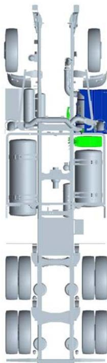
The SCR system components are integrated with the vehicle chassis. Vehicle packaging for these components is dependent upon exhaust configurations specified and the application. For example, in a typical vehicle, the DPF and SCR catalysts will most likely be positioned within the toolbox mounted under the cab as illustrated in blue in the rendering at left.
